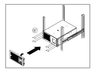
**CAUTION!** The UPS must be installed at the bottom of the rack system. **CAUTION!** Do not lift the front panel when removing the UPS unit.
